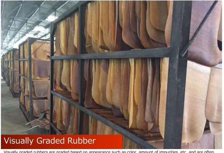
Visually graded rubbers are graded based on appearance such as color, amount of impurities, etc. and are often used in tires, anti-vibration rubber, and other mold items. We offer a wide range of visually graded rubbers from most major producing countries which are delivered to you in sizes ranging from 20kg to 113kg per bale.
