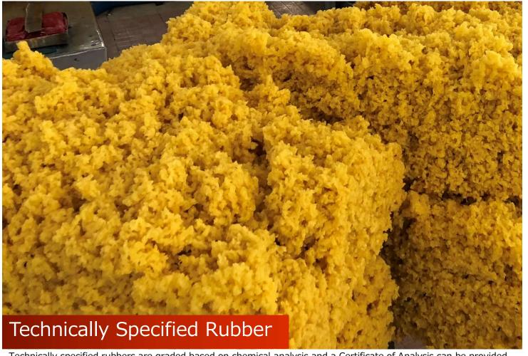
Technically specified rubbers are graded based on chemical analysis and a Certificate of Analysis can be provided to show the test results of their physical properties. They are used in a wide range of rubber products from tires to adhesives. We are able to provide TSR rubber from Thailand, Vietnam, Malaysia and more, in bale form.
